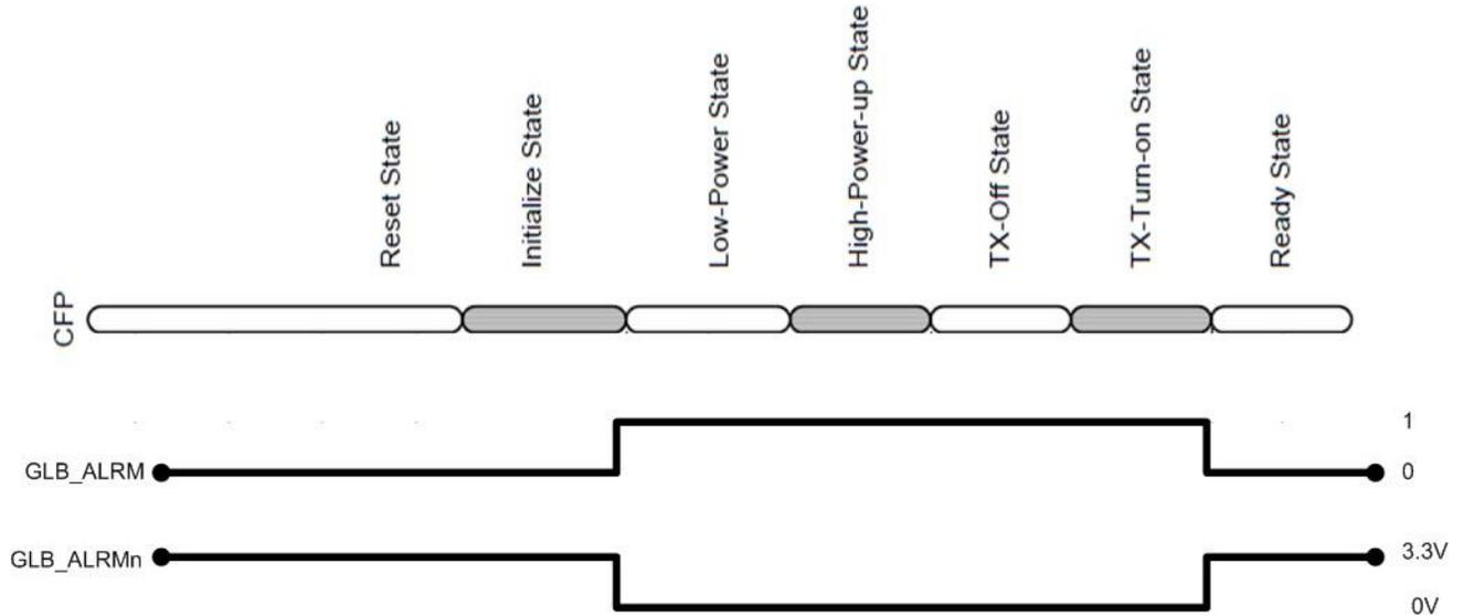
GLB\_ALARM is de-asserted during Reset and Initialize state, it is asserted in Low-Power, High-Power-up, Tx-Off and TX-Turn-on states, then de-asserted again when ready state is reached. GLB\_ALRMn is the hardware pin, and is the inverse of GLB\_ALARM.
