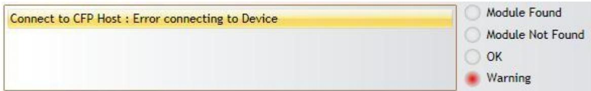
**Figure 12 Communication status box showing a connection error**
